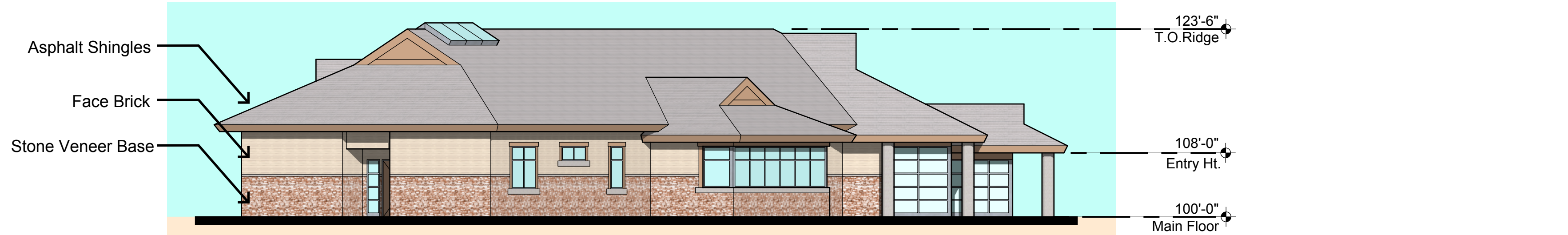
(B) 3 EAST ELEVATION Scale: 3/32" = 1'-0"
