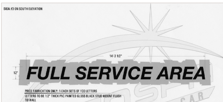
5 9 DETAIL BUILDING WALL SIGN NTS
