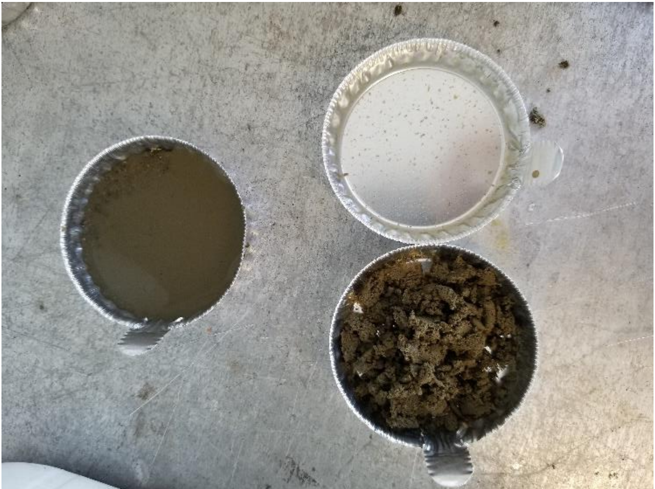
Figure 3: Influent sludge (Left) compared to the cake solids (Bottom Right) and pressate (Top Right).
