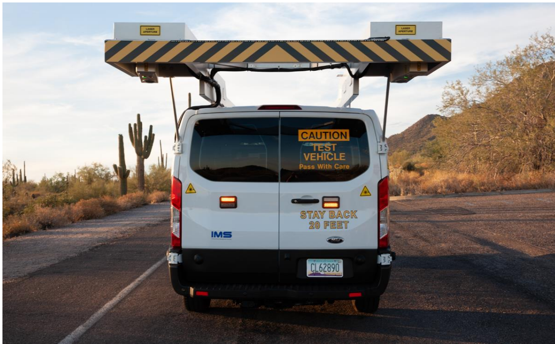
Figure 9 - LCMS2 data collection vehicle
