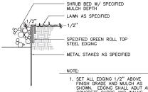
1. SET ALL EDGING 1/2" ABOVE FINISH GRADE AND MULCH AS SHOWN. EDGING SHALL ABUT ALL CONCRETE CURBS AND WALKS PERFENDICULAR AND FLUSH W/ GRADES OF CONCRETE. ALL JOINTS TO BE SECURELY STAKED.
