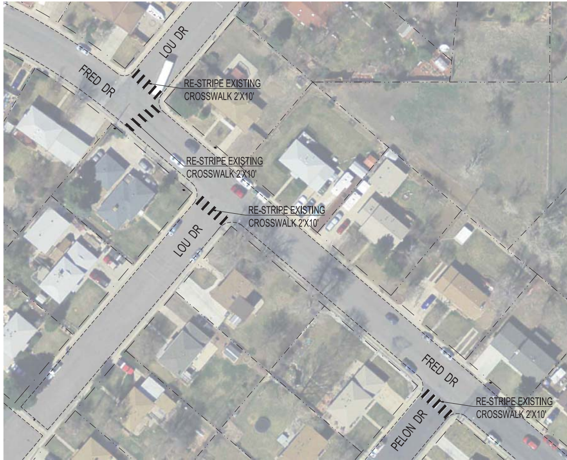
BID ALT - CROSSWALK STRIPING INTERSECTIONS
