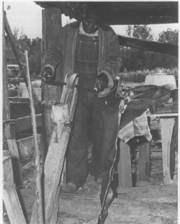
5. Custom Handsplit shingles are still made the traditional way with a mallet and froe or ax. For these cypress shingles, a "bolt" section of log (photo A) the length of the shingle has been sawn and is ready to be split into wedge-shaped segments. Handsplit shingles are fabricated with the ax or froe cutting the wood along the grain and separating, or riving, the shingle away from the remaining wedge. The rough surfaces are dressed on a shavinghorse using a draw-knife as shown above (photo B). Note the long wooden shingles covering the work shed in photo A. Photos: Al Honeycutt, North Carolina Division of Archives and History.
