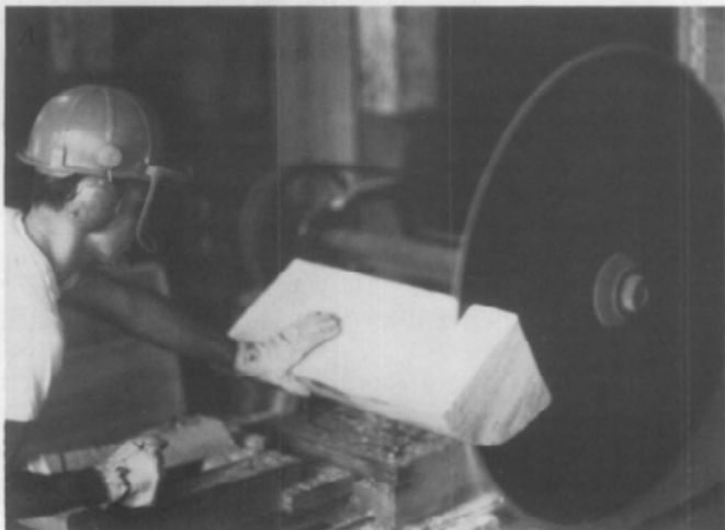
6. Modern machine-made shingles are sawn. Shown are: (photo A) Eastern White Pine quarter split shingle block on equalizer saw being trimmed to parallel the ends; and (photo B) the restored 19th-century shingle mill saw cutting tapered flitches or shingles. The thickness and taper can be precisely controlled. Photo: Steve Ruscio, The Shingle Mill.
