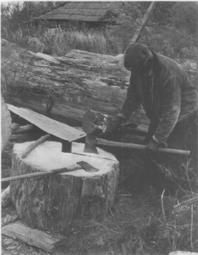
5. Custom Handsplit shingles are still made the traditional way with a mallet and froe or ax. For these cypress shingles, a "bolt" section of log (photo A) the length of the shingle has been sawn and is ready to be split into wedge-shaped segments. Handsplit shingles are fabricated with the ax or froe cutting the wood along the grain and separating, or riving, the shingle away from the remaining wedge. The rough surfaces are dressed on a shavinghorse using a draw-knife as shown above (photo B). Note the long wooden shingles covering the work shed in photo A. Photos: Al Honeycutt, North Carolina Division of Archives and History.
