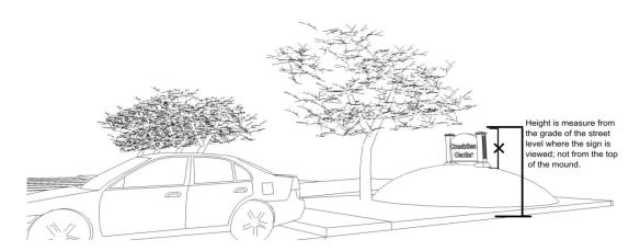
B. Clearance for freestanding and projecting signs shall be measured as the smallest vertical distance between finished grade and the lowest point of the sign including any framework or other embellishments.
