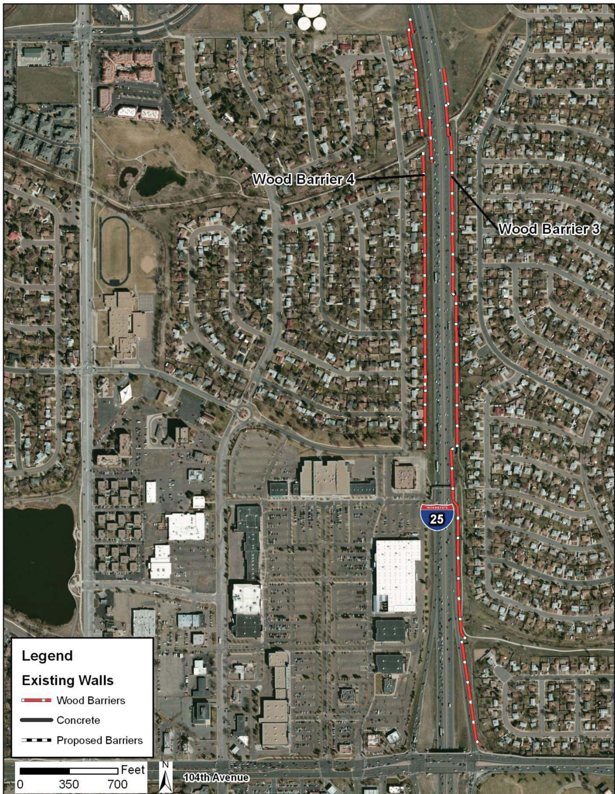
Exhibit 4. Existing Wood Noise Barriers 3 and 4
