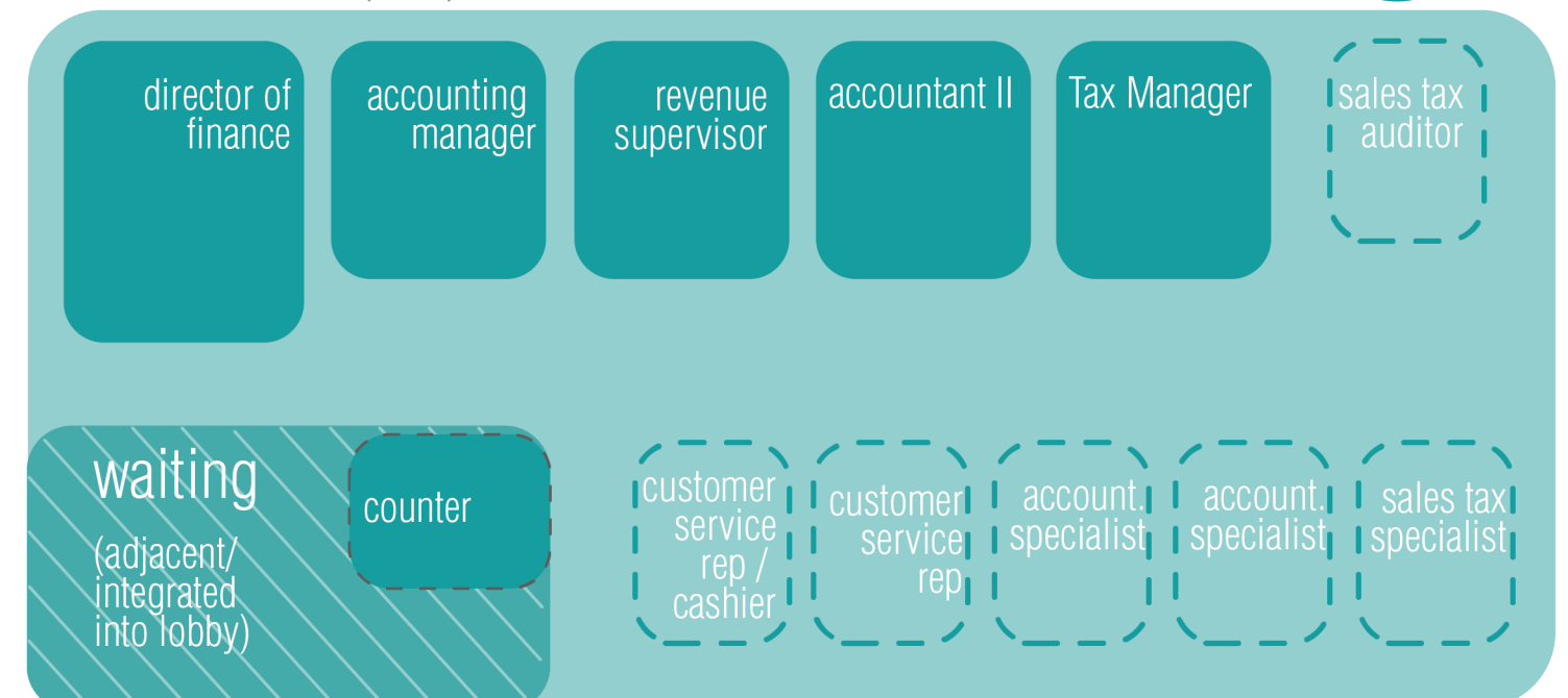
Figure III.7 - Graphic Program Summary of Finance Department and relationship between individual offices and workstations
